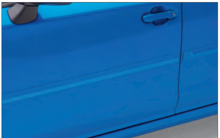
Body Side Molding. Attractive, color-matched moldings coordinate with the styling of the vehicle while helping to protect doors from unsightly dings.
